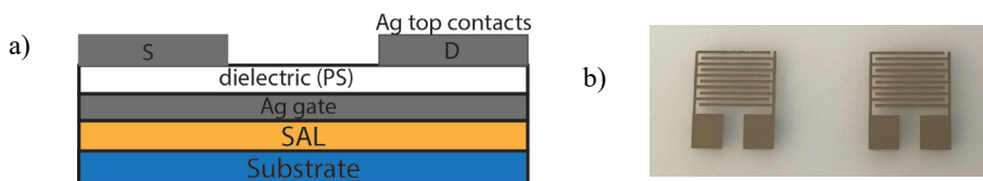
Fig. 1. Schematic representation of selected PPFET's architecture (a) and photo of the screen-printed source and drain electrodes (b).
