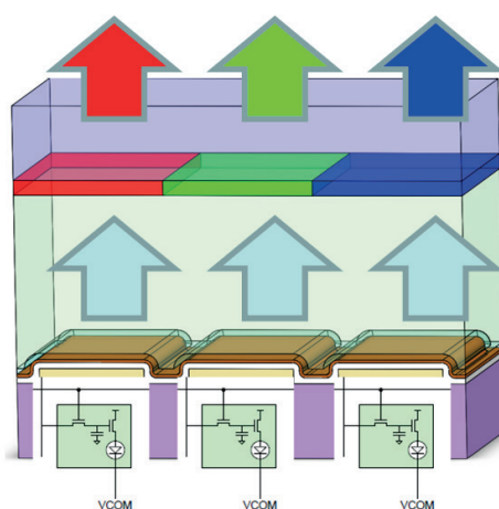
Fig. 1. Full color display pixel based on initial white OLED and RGB filter matrix.
